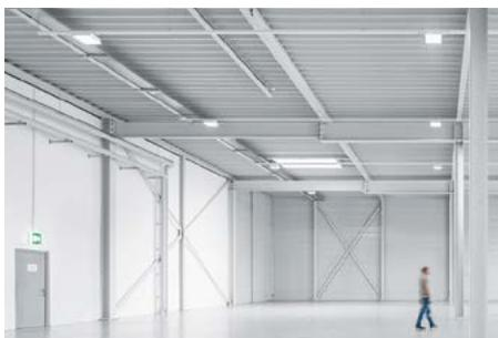
High-bay LED luminaires installed on TECTON trunking can be easily relocated, if required.
