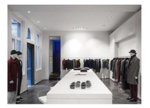
**Image 2:** The white driver modules of the INTRO system fit adroitly into the ceiling, helping to ensure sufficient general lighting and to focus attention on the latest collections.
