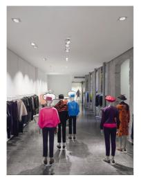
**Image 3:** Each dummy is highlighted by a pair of accent spotlights from the INTRO lighting system, which is fitted flush into the ceiling. One spotlight with a focused distribution and one with floodlight characteristics offer the optimal combination.
