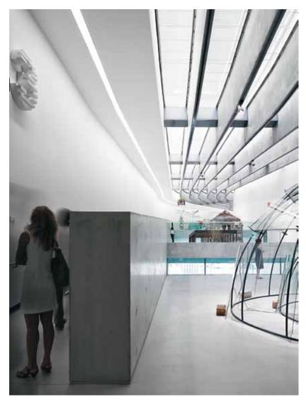
B6 I All the technical elements are accommodated in the complex luminous ceilings. The general illumination is provided by light bands with dimmable fluorescent lamps fitted behind light-scattering translucent acrylic glass. Spots offer additional point illumination.
