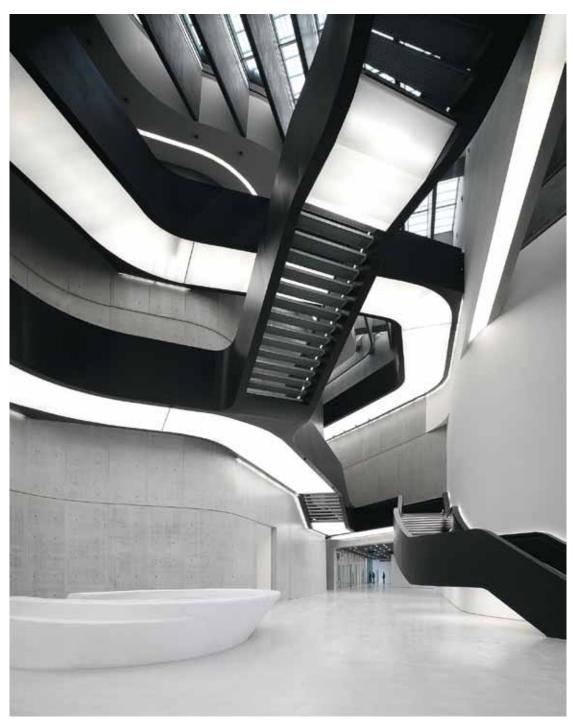
B2 I The soft light not only radiates downwards, but also diffuses upwards through the grating of the steps and pathways. Light bands hidden in the handrails follow the stairs as a source of indirect illumination.
