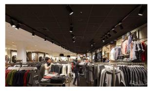
young fashion accessories, appealingly and to full effect. Zumtobel used its latest lyon LED spotlight range and its Cardan LED lighting system to satisfy this requirement. The lyon spotlight's sophisticated design accommodates a unique lens/reflector system that allows for high-precision, homogeneous accent lighting with a variety of beam patterns. With a stable warm white colour temperature of 3000 K and excellent colour rendering (Ra > 90), the LED
