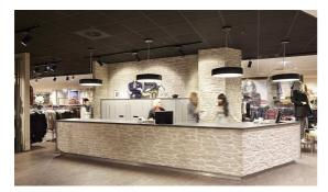
In the checkout areas, care was also taken that the luminaire design matches the interior and provides homogeneous ambient lighting. As in the entrance area, round pendant luminaires are used above the checkout counters. In order to
