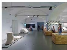
**Fig. 2:** On a floor space of 2000 square metres, some 300 DISCUS evolution LED spotlights – instead of 100 halogen spotlights with low efficiency – ensure individual presentation of approximately 2000 exhibits.
